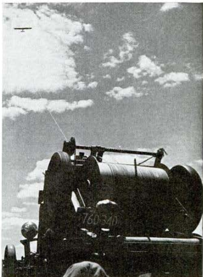
Power winch used to launch sailplanes. High in the sky is a sailplane whose pilot has not yet cast off the tow line
